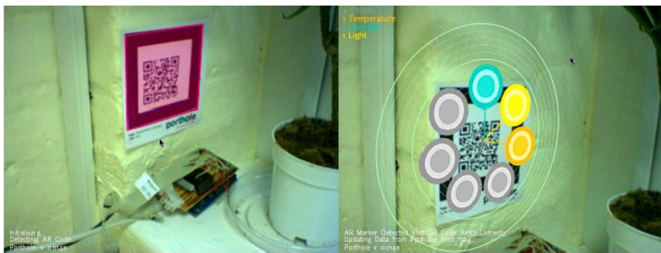
Porthole marker corresponding to a networked sensor device is detected – several datastreams are discovered
